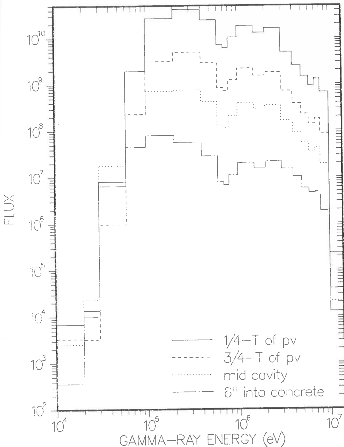
Fig. 5.20 Gamma energy spectra [ \gamma \cdot \text{cm}^{-2} \cdot \text{s}^{-1} ] at four radial locations throughout the RPV and the concrete shield wall at the axial core mid-plane
